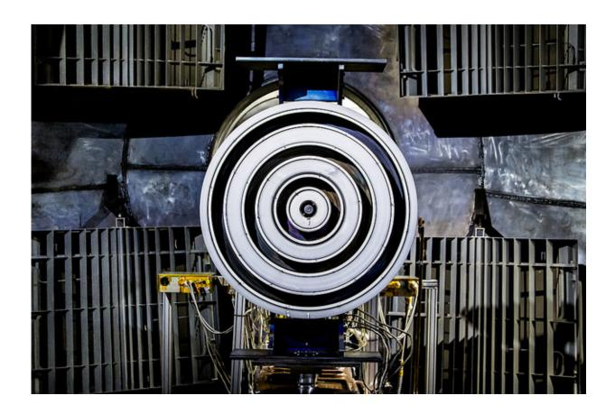
An X3 thruster that AERO Professor Alec Gallimore's team has been working on in conjunction with NASA in the Plasmadynamics & Electric Propulsion Laboratory in Ann Arbor, MI on April 28, 2015. The thruster is being built and tested with hopes of it powering humans to Mars in the near future. Credit: Joseph Xu, Michigan Engineering Communications & Marketing
