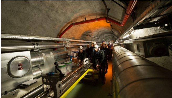
AWAKE's 10-metre-long plasma cell developed by MPP has been moved into place in the experiment tunnel. Credit: Maximilien Brice/CERN
