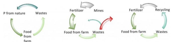
Original phosphorus cycle (left); the broken cycle (centre); and an optimised cycle (right).
