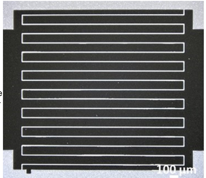
A supercapacitor under an optical microscope. To optimize space, its 18 electrodes are interdigitated. Credit: CIRIMAT
