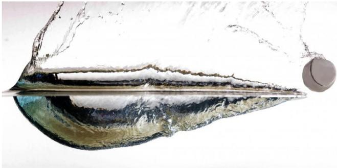
A high-speed camera captured this image of an elastic sphere bouncing off the water surface in a tank. Credit: Chris Mabey
