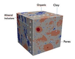
X-ray microscopy (XRM) image of an untreated sample of gas shale, showing inclusions of pyrite, clay, organic matter and other minerals. Credit: M. Hubler (MIT) and J. Gelb (Carl Zeiss X-ray Microscopy)
