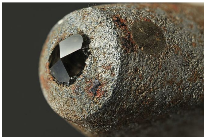
Vickers test anvil. Credit: R Tanaka, CC BY
