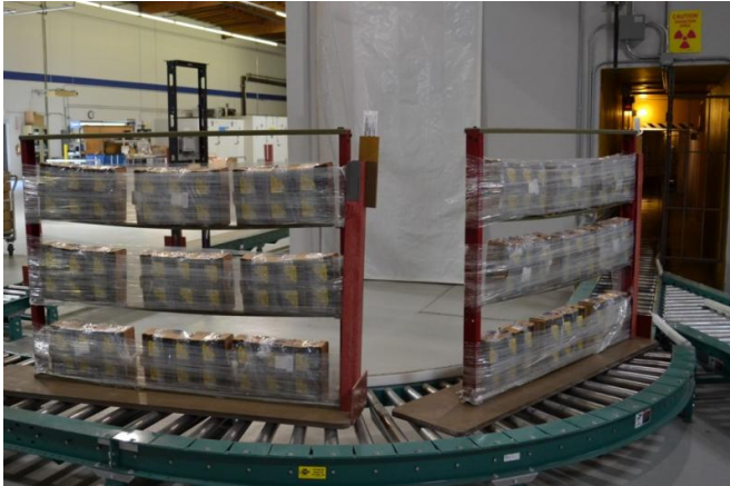
Blueberries ready to enter the x-ray unit at the irradiation facility. Credit: Photo courtesy of Anuradha Prakash.
