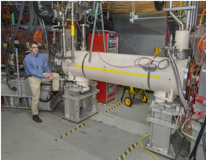
Brookhaven Lab accelerator physicist Wolfram Fischer stands next to the electron lensing apparatus at the Relativistic Heavy Ion Collider (RHIC), a particle accelerator/collider at the US Department of Energy's Brookhaven National Laboratory. Credit: Brookhaven National Laboratory
