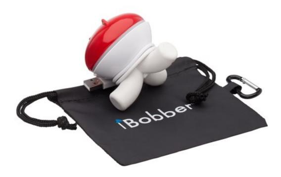
This undated photo provided by ReelSonar shows the iBobber. The iBobber fish finder attaches to your fishing line and floats on the surface of the water. Once you cast it, the iBobber can show you where fish are and how big they are. It also maps the floor of the waterbed, letting you know how deep the water is and pointing out obstacles, as far down as 135 feet, whether you fishing from shore, boat or dock. (ReelSonar via AP)
