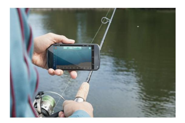
This undated photo provided by ReelSonar shows someone demonstrating the use of the iBobber. The iBobber fish finder attaches to your fishing line and floats on the surface of the water. Once you cast it, the iBobber can show you where fish are and how big they are. It also maps the floor of the waterbed, letting you know how deep the water is and pointing out obstacles, as far down as 135 feet, whether you fishing from shore, boat or dock. (Meagan
