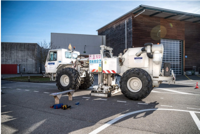
A seismic truck at Point 1 generated wave-like vibrations measured by EN/MME. Credit: Sophia Bennett/CERN
