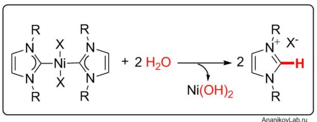
Hydrolysis of the Ni-NHC complexes leading to the release of Ni hydroxide and free ligand. Credit: AnanikovLab
