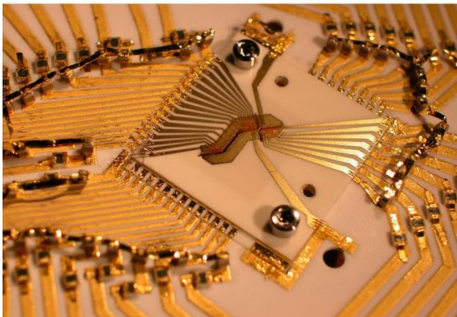
An ion trap used in NIST quantum computing experiments demonstrating logic operations with two different types of ions (charged atoms). One magnesium ion and one beryllium ion are trapped 4 micrometers apart near the cross-shaped opening at the center of both photos. The larger-scale photo shows the gold-on-alumina trap inside a case that protects against electrical interference. Credit: Blakestad/NIST
