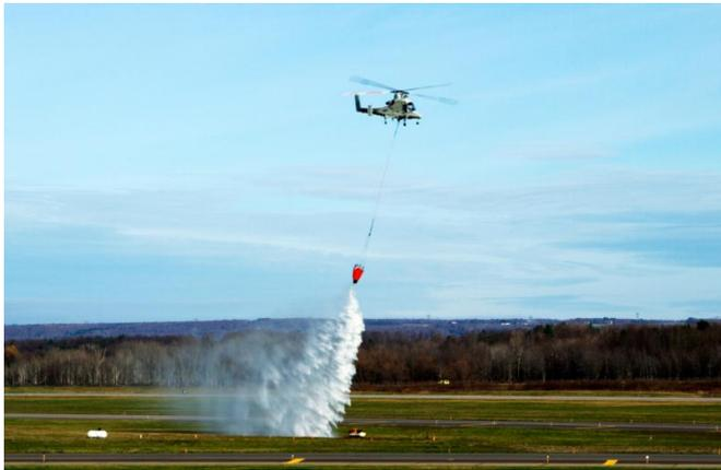
The Stalker UAS directs the unmanned K-MAX cargo helicopter to conduct water drops at a precise location to extinguish a fire. The Stalker and K-MAX operated in collaboration with a prototype UAS Traffic Management (UTM) system, which provides essential capabilities to enable safe UAS operations.
