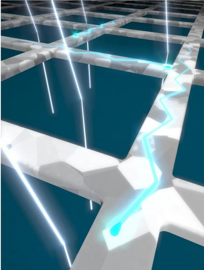
The image shows a network of silver nanowires created with the new technique. The white lines running from top to bottom represent rays of light, which move in a straight line through the lattice. The blue lines are the electrons that cannot pass straight through, because they are scattered at the boundaries between the silver crystals. Individual crystals are visible via the colour contrast. Credit: Henk Jan Boluijt/AMOLF
