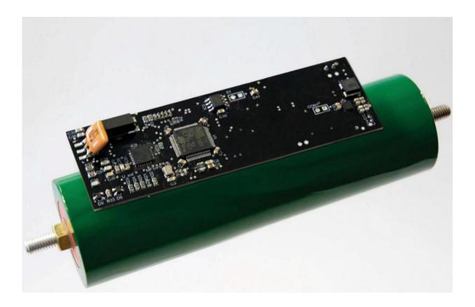
Intelligent cell of the Fraunhofer IPA: A microcontroller records physical parameters such as temperature and state of charge. If a cell is empty, it switches itself off automatically. Credit: Fraunhofer IPA
