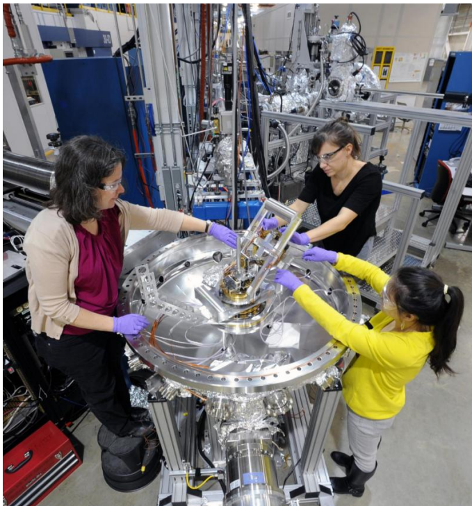
Clockwise: Jessica McChesney, Fanny Rodolakis, and Yizhi Fang installing the in-vacuum kappa diffractometer into the resonant soft X-ray scattering endstation
