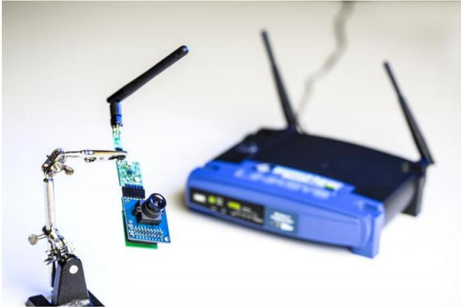
The UW team used ambient signals from this Wi-Fi router to power sensors in a low-resolution camera and other devices. Credit: Dennis Wise/University of Washington
