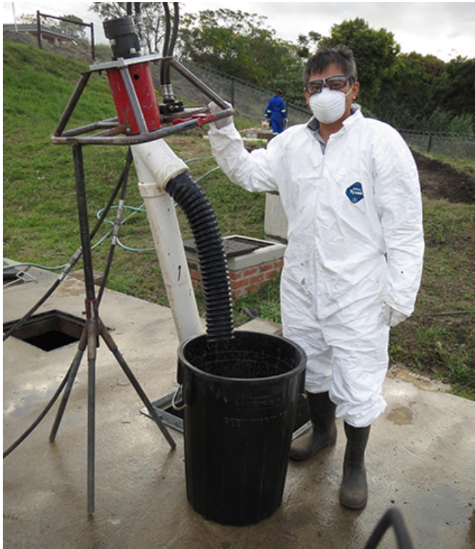
De los Reyes testing an early version of the "Excrevator" in South Africa. Credit: of Francis de los Reyes
