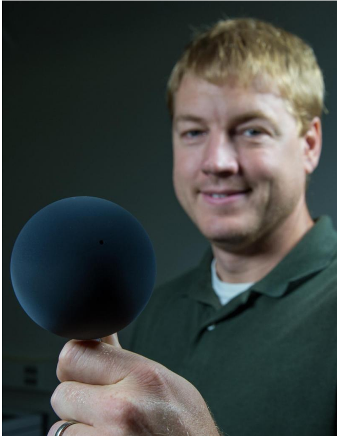
Principal Investigator Phillip Chamberlin holds a sphere coated in super-black carbon nanotubes. Credit: NASA/W. Hrybyk
