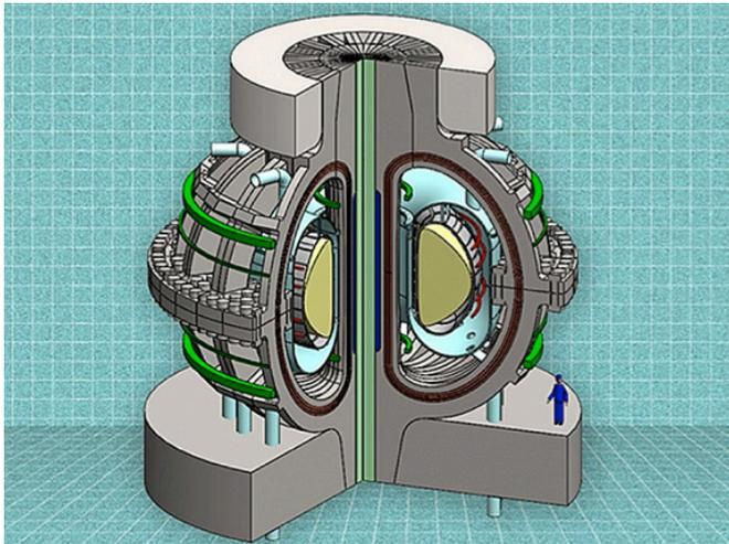
Conceptual design of the ARC fusion reactor. About the same size as the currently operating JET tokamak in the United Kingdom, but with three times the magnetic field strength, ARC is sized to produce 500 MW of deuterium-tritium fueled fusion power. Credit: Earl Marmor
