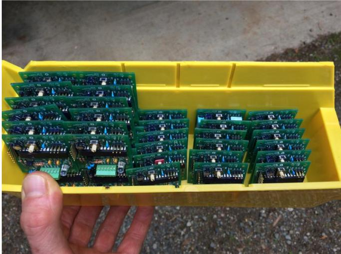
40 control boards ready to be attached to battery packs.
