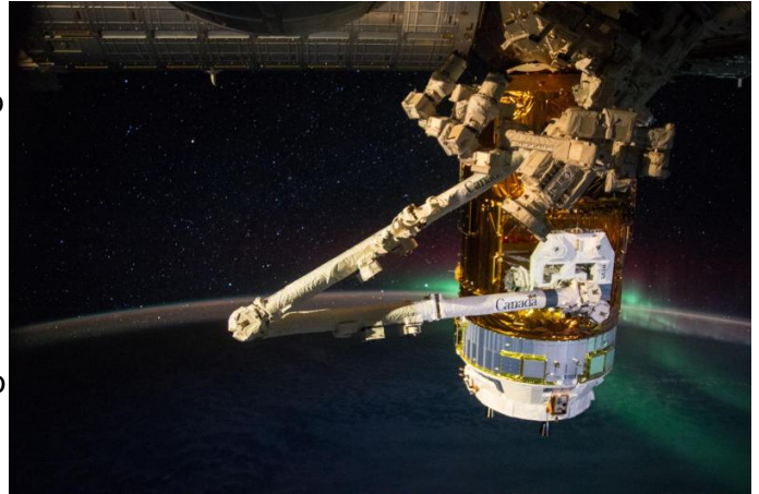
The Japan Aerospace Exploration Agency (JAXA) Kounotori H-II Transfer Vehicle (HTV-5) is seen berthed to the International Space Station. The external CALET experiment, which will search for signatures of dark matter, is seen being extracted from the unpressurized section by the station's robotic arm, Canadarm2. An aurora over the Earth limb is visible in the background. Credit: NASA
