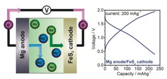
The electrolyte—the electrically conducting component—contains sodium and magnesium ions. Testing showed that the resulting device's energy density was close to that of <a href="lithium-ion batteries">lithium-ion batteries</a>. It could get an additional two- to three-fold boost with further development of magnesium electrolytes. And because it's made with low-cost materials, it could one day help support grid-scale energy storage, the researchers say.
