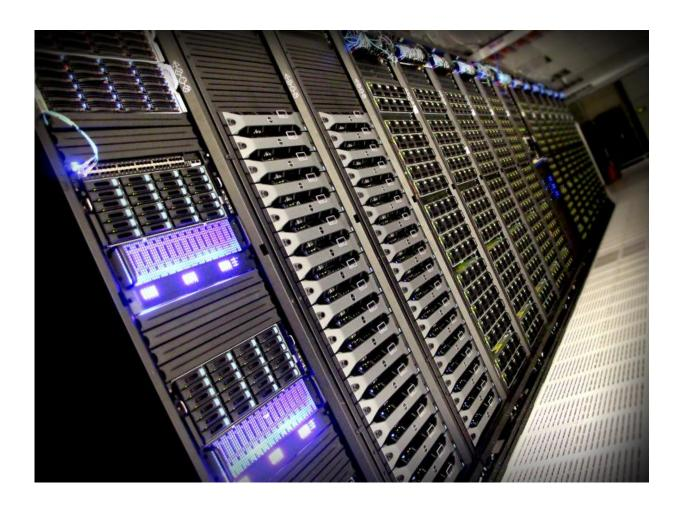
SDSC's new Comet supercomputer, a petascale cluster funded by the NSF, is designed to run as many as 10,000 research jobs simultaneously. Credit: Ben Tolo, SDSC
