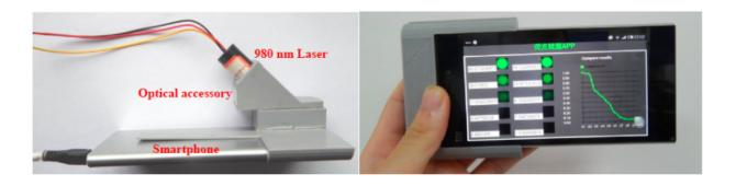
The prototype smartphone-based detection system – courtesy of Professor Mei et al., the images first appeared in the paper in *Biosensors and Bioelectronics*.
