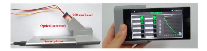
The prototype smartphone-based detection system – courtesy of Professor Mei et al., the images first appeared in the paper in *Biosensors and Bioelectronics*.
