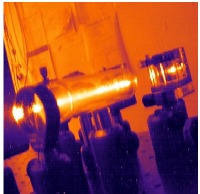
Infrared image of a laser probing a Caesium vapour cell. Credit: GW Truong
