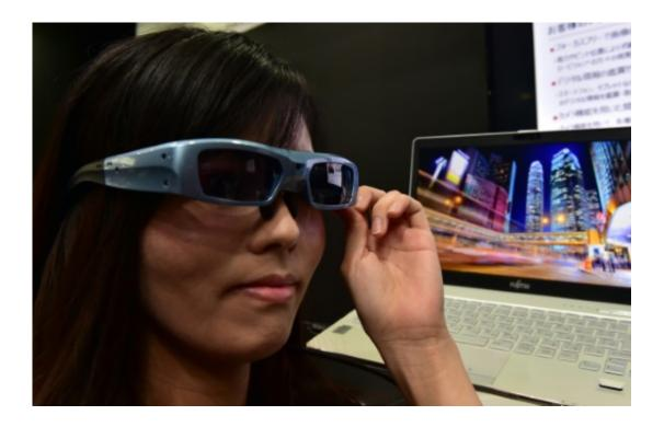
An employee of Japan's computer giant Fujitsu demonstrates a prototype of the 'Retissa' retinal imaging eyewear - which can project digital images onto the user's retina using laser beams, at CEATEC, in Chiba, suburban Tokyo, on October 7, 2015
