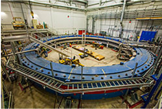
The superconducting magnet of the Muon g-2 experiment.
