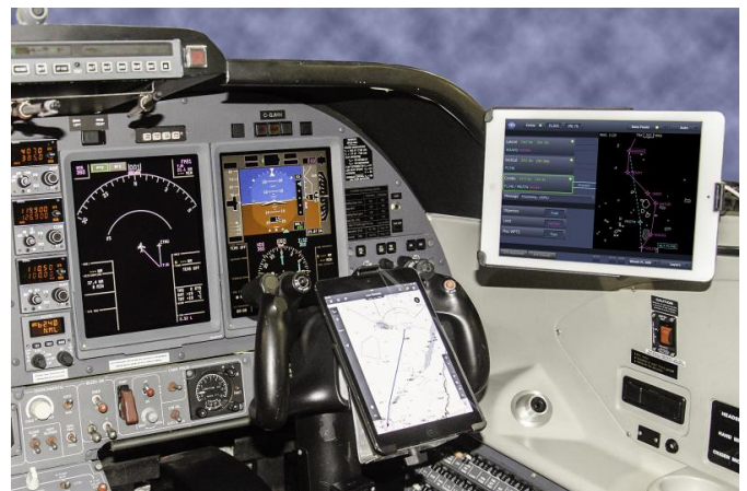
The TASAR application can be seen in the far right screen. Credit: NASA/David C. Bowman
