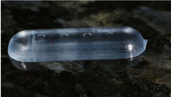
Plastic prototype pill with indentations of less than 0.5mm, creating a 3-D barcode. Credit: Ben Whiteside, University of Bradford
