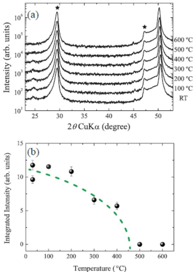
The x-ray diffraction patterns with inclination angle of 45° observed for 0.07YO<sub>1.5</sub>-0.93HfO<sub>2</sub> film measured from room temperature to 600° C. (b) The integrated intensity of the 111 super-spot of 0.07YO<sub>1.5</sub>-0.93HfO<sub>2</sub> film as a function of temperature.
