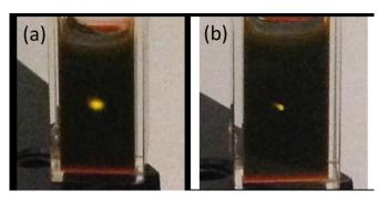
Photographs of upconversion in a cuvette containing cadmium selenide/rubrene mixture. The yellow spot is emission from the rubrene originating from (a) an unfocused continuous wave 800 nm laser with an intensity of 300 W/cm2. (b) a focused continuous wave 980 nm laser with an intensity of 2000 W/cm2. The photographs, taken with an iPhone 5, were not modified in any way. Credit: Zhiyuan Huang, UC Riverside.
