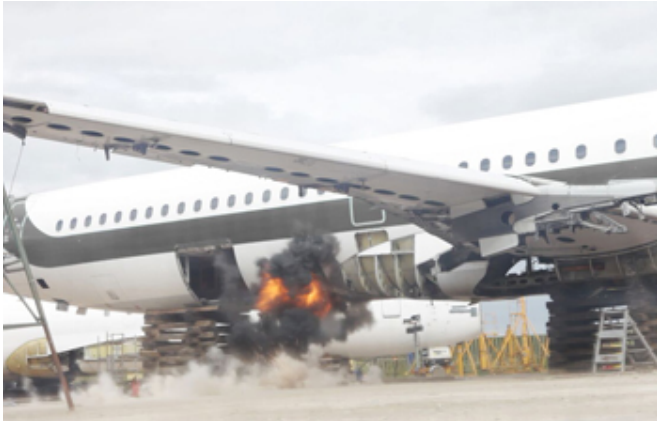
A controlled explosion without Fly-Bag in the hold. Credit: University of Sheffield
