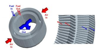
A heat exchange device developed at Purdue University could help cool supersonic engines in aircraft and maintain acceptable temperatures to operate at optimum speeds. The technology uses the aircraft's own fuel to cool the compressor air before it is used on hot engine components. The technology was developed by Issam Mudawar, professor in Purdue's School of Mechanical Engineering and is patented through the Purdue Office of Technology Commercialization. Credit: Purdue University
