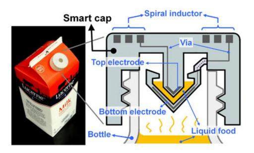
UC Berkeley engineers created a 'smart cap' using 3D-printed plastic with embedded electronics to wirelessly monitor the freshness of milk. Credit: Sung-Yueh Wu
