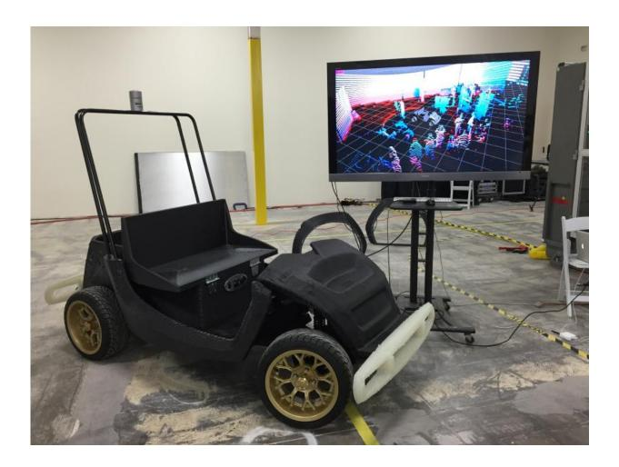
A fleet of autonomous "SmartCarts"-high-tech, 3D-printed, low-speed
