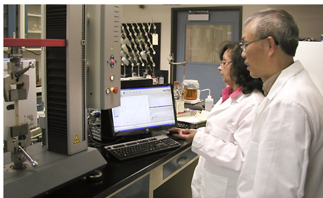
ARS chemists Dorselyn Chapital (left) and Zhongqi He use a testing device to measure the shear strength of an adhesive bond between two pieces of wood. Credit: Mary Lovisa and Kelly Williams
