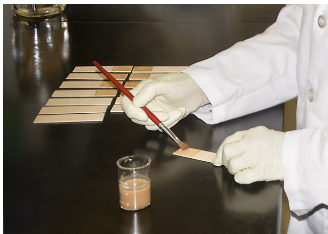
Washed cottonseed meal adhesive being applied onto one end of a pair of wood strips that will be bonded by hot-pressing. Credit: Mary Lovisa and Kelly Williams
