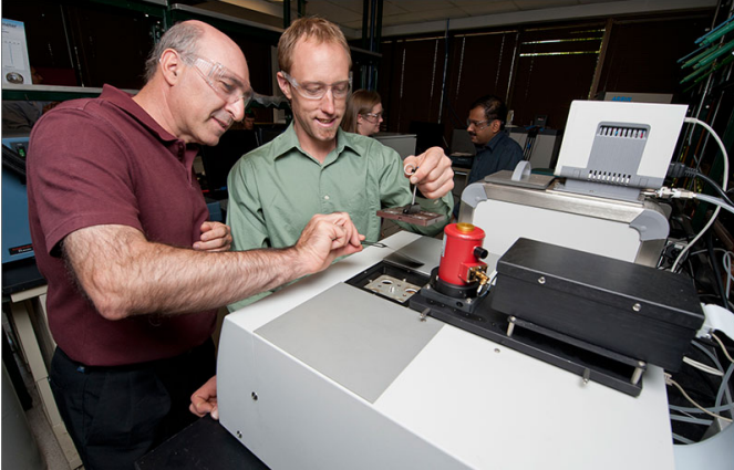
NREL researchers Ahmad Pesaran, left, and John Ireland work on a cell calorimeter at the Battery Testing Laboratory. Credit: Dennis Schroeder
