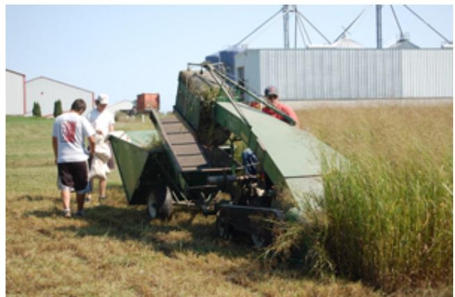
Harvesting switchgrass biomass samples with a flail harvester. Machine cuts and picks up biomass, blows it through a chute, weighs the biomass, and dumps in a wagon. Students pull random samples for dry matter determination. Credit: M. Casler
