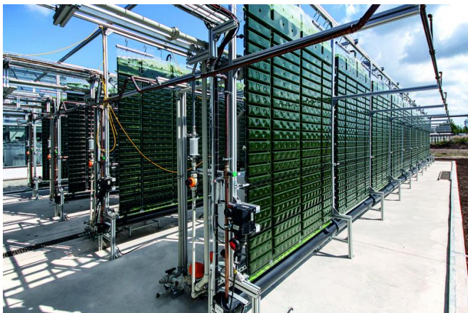
180-liter reactor module installed at Fraunhofer CBP's outdoor facility in Leuna. Credit: Fraunhofer IGB
