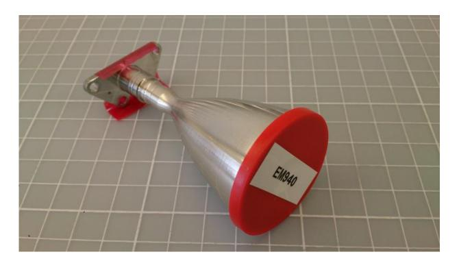
The combustion chamber and nozzle for the 10 N hydrazine thruster were printed in platinum–rhodium alloy using a laser beam applied to a metal powder bed. A hot firing campaign followed, reaching a maximum throat temperature of 1253°C. The prototype thruster was produced and tested at the Airbus Defence & Space facility in Lampoldshausen, Germany, through an ESA project called Additive Manufacturing Technologies for Advanced Satellite Thrust Chamber, AMTAC. Credit: Airbus Defence & Space
