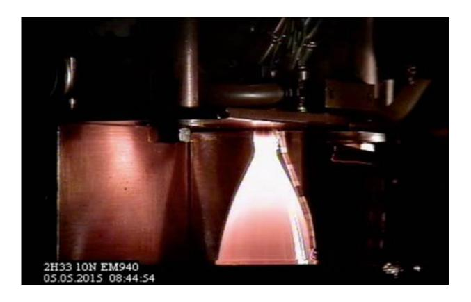
The world's first spacecraft thruster with a platinum combustion chamber and nozzle made by 3D printing has passed its baptism of fire with a series of firings lasting more than an hour and 618 ignitions. The firings included a single burn of 32 minutes, during which a maximum throat temperature of 1253°C was attained. Credit: Airbus Defence & Space
