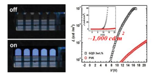
Electroluminescent images of GQD-LEDs (left) and luminescence efficiency of GQD-LEDs (right). Credit: KAIST
