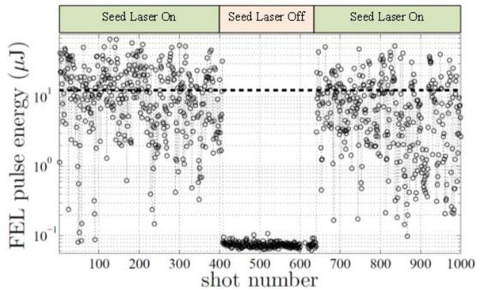
The plot for experts: In HGHG mode, the pulses of radiation inside the sFLASH undulator, which is just ten metres long, have mean energies of over 10 microjoules ( $\mu\text{J}$ ), whereas the “normal” SASE intensity observed when the laser beam is switched off is a factor of about a thousand lower.
