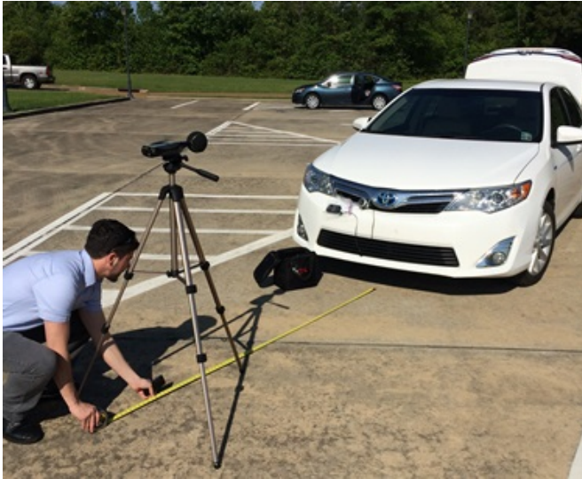
Louisiana Tech researchers conduct noise output measurements on electric cars. Credit: Louisiana Tech University
