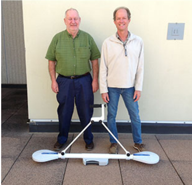
Stephen Ackley and Blake Weissling show the new Electromagnetic Induction Meter that will be used in the Arctic in October. Credit: Kris Rodriguez
