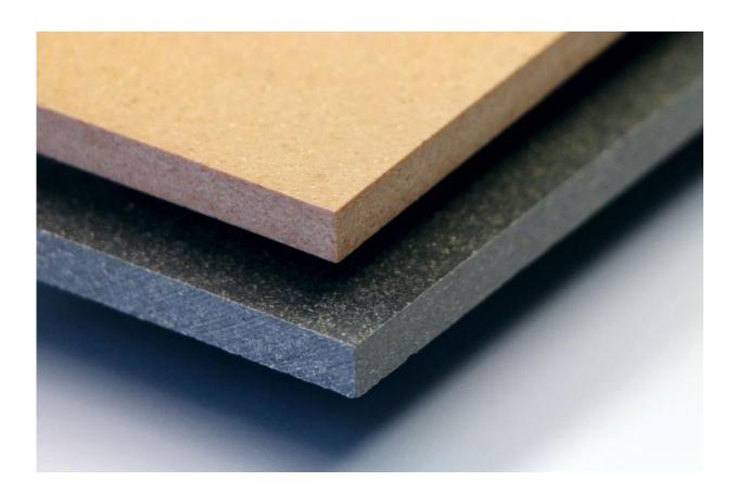
WPC board without (above) and with (below) flame-proofing. Credit: Fraunhofer WKI
