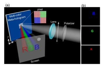
The multicolor meta-hologram is made of a pixel array consisting of aluminum nanorods of different lengths that produce different colors of light. Credit: Huang, et al. ©2015 American Chemical Society
