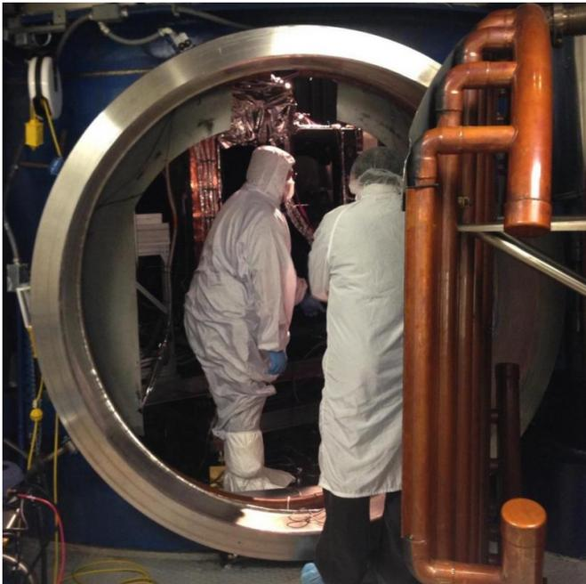
The door of a thermal vacuum chamber at NASA's Goddard Space Flight Center in Greenbelt, Maryland, closed behind the ATLAS box structure (an instrument for the ICESat-2 mission) on Feb. 5, 2015, after final checks from the thermal, electrical, fiber-optics, mechanical, contamination, instrument and quality assurance teams, among others. Credit: NASA Goddard/Kate Ramsayer
