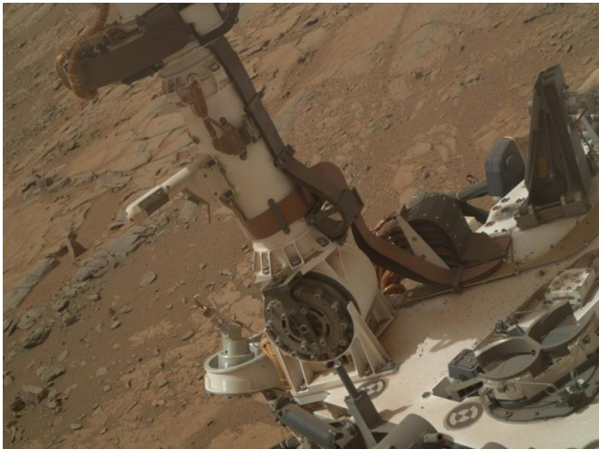
Mast and rover deck where the REMS air and ground temperature (boom), and UV sensors are located (sol 177). Credit: NASA/JPL-Caltech/MSSS
